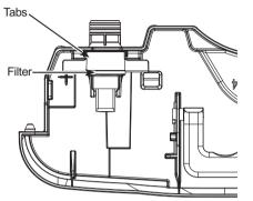
**IMPORTANT:** Be careful not to tear or damage filter during removal, cleaning or replacement. Do not use the dishwasher to clean the filter.
