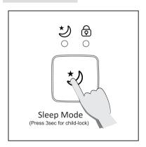
\*Press Sleep button ,air purifier will enter into sleep mode ,the indicator light of sleep mode will be on ,the fan speed and noise level will change to the lowest,all the indicators will be off ,exist the sleep mode function by pressing any button , except the ON/OFF button.
