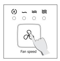
After plugged in the power ,the air purifier enters standby mode .Press ON/OFF button, then the air purifier will on and enter AUTO mode,under this mode ,the air purifier will choose wind speed automatically according to the air quality.
