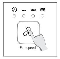
Under manual mode, you can choose the wind speed through FAN SPEED button, there are three gears of wind speed: gear1, gear 2, gear 3 and auto mode.
