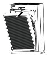
6. To reinstall the back cover, align and insert the fixed groove, then exert pressure at top of the machine, and fix the back cover to be close to the magnetic door holder
