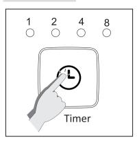
Timer is much convenient for you to control the air purifier. You can set up the working hour of the air purifier by 1 hour 2 hours 4 hours 8 hours.
