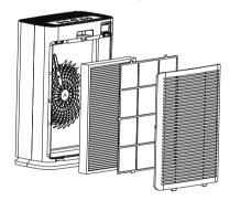
4. Remove the bag on filter net.
