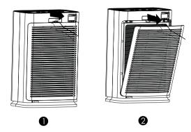
3.Remove the filter assembly inside the purifier. (Tips: Remove the filter assembly follow the arrow direction).
