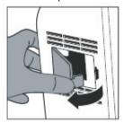
3. Use wet cotton stick to clean air quality sensor, air inlet and air outlet.
