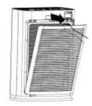
4. Remove partcles with sof brush or vacuum cleaner. Clear the filter net with water and mild soap-suds and put the filter net into machine after it is completely dry.
