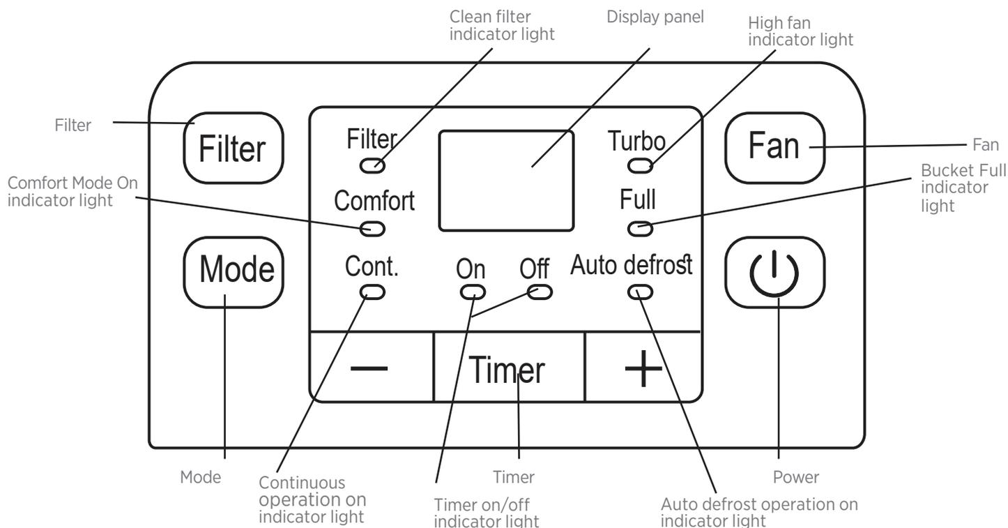
**Power:** Press to turn the dehumidifier on and off.
