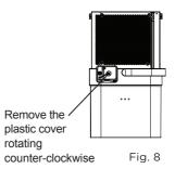
When removing the drain hose, some water may remain in the hose or the drain outlet. Be sure this water will not spill by drying the wet area before moving the unit.
