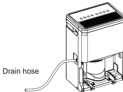
3. Thread a garden hose (not supplied) onto the nozzle and ensure it is seated securely. Cut to length and lead it to the floor drain.
