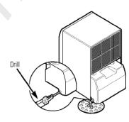
**NOTE:** The nozzle cannot be fixed after puncture. Use an ordinary garden hose cap (not included) to reclose if necessary.
