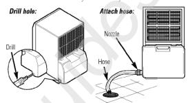
**3 Use a floor drain.** The unit can also be placed over a floor drain. Using a drill, make a hole at the end of the nozzle located on the lower left side of the bucket.
