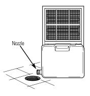
**NOTE:** The nozzle cannot be fixed after puncture. Use an ordinary garden hose cap to reclose if necessary.
