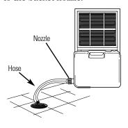
**3 Use a floor drain.** The unit can also be placed over a floor drain. Using a drill, make a hole at the end of the nozzle located on the lower left side of the bucket.
