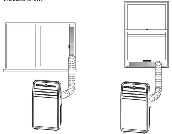
**Note**: For optimum performance, make sure the venting hose is not twisted and is free of kinks. For better efficiency, shorten the hose by squeezing its sections together.
