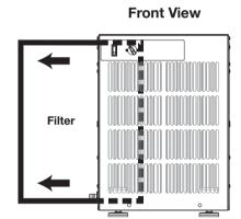
**Step 3 -** Insert the new filter into the filter compartment and attach the magnetized filter door back into place, ensuring it covers the filter compartment completely. Be sure the arrows on the filter are facing into the dehumidifier.
