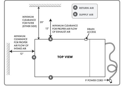
• Electrical service access will require the removal of the rear panel where the power cord is located. Allow sufficient clearance around the unit.
